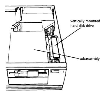
2. Remove the retaining screw securing the hard disk drive mounting plate to the computer and set it aside.
